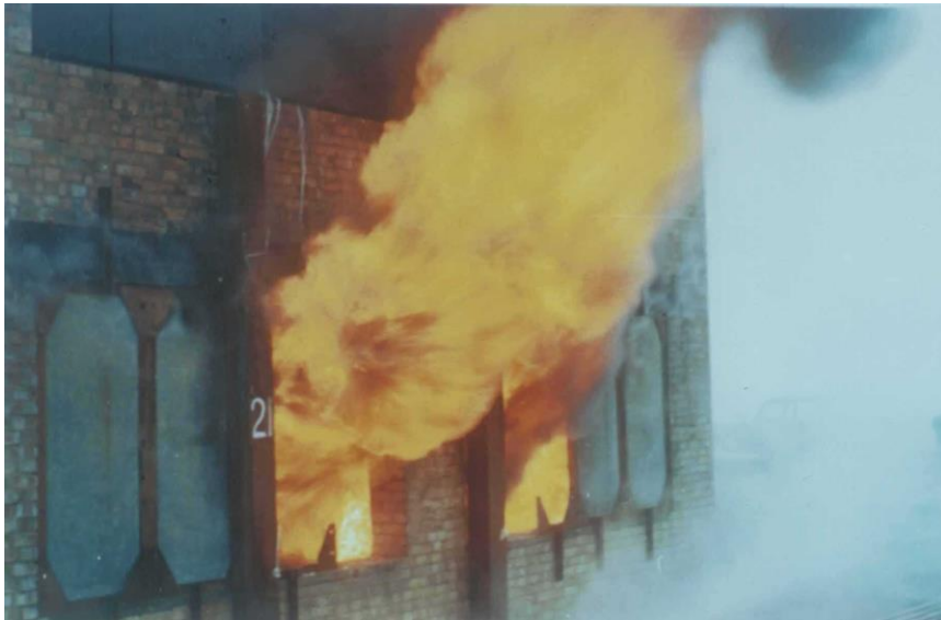
Ventilation controlled fire. Fuel load, fibre insulation board, 7.5 kg/m 2
