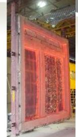
Horizontal Furnace capable to test loadbearing building elements
