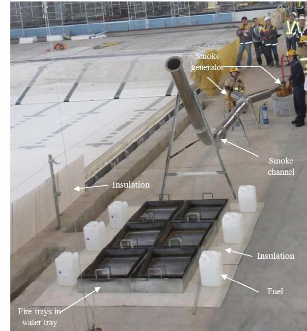
Typical Indicative Set-up for Hot Smoke Test
