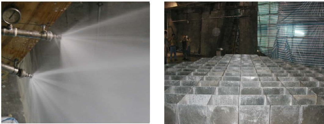
Figure 8: Field Test of Long Throw Sprinkler with 30° and 45° inclined
